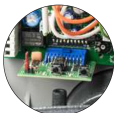
SCHEDA RADIO RICEVENTE OPEN COLLECTOR
