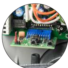
SCHEDA RADIO RICEVENTE OPEN COLLECTOR
